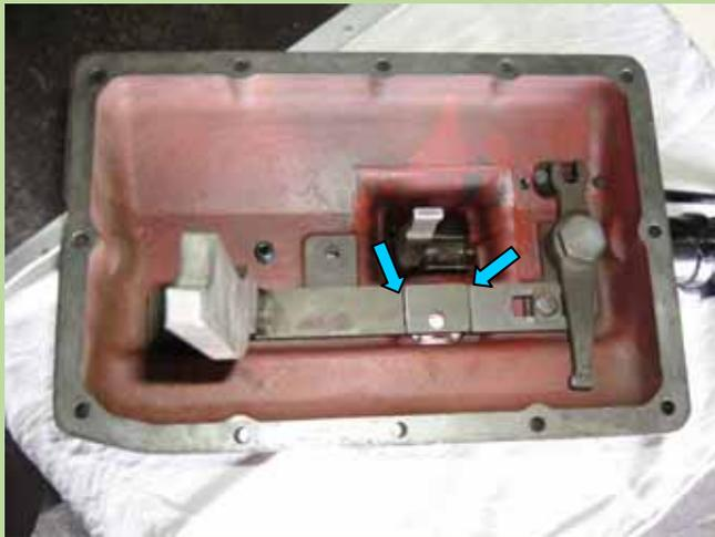
When the shifting fork is apart, mark 75mm (from the right to left) and a second segment of 40mm. Cut the pieces and eliminate sharp edges, sand them. This pieces are for the connection of the new shift lever with the high/low range slider on the shift plate.
