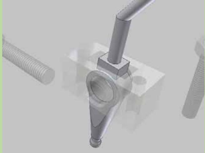
The new finger fit into the receiver on the main shift plate (yellow arrow), This must be measured and arranged on the shift plate and then welded.
