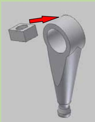
←----- Weld the receiver part to the (70mm) shift finger
